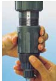
The injection rate is set by lining up the top of the adjusting sleeve with the desired ratio on the scale. The amount of injected concentrate is proportional to the amount of water coming into the Dosatron : i.e. Adjustment at 1% = 1 : 100 = 1 Volume of concentrate into 100 Volumes of water.
